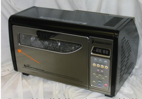
Remove right and left side panels : 6 screws right side- 7 screws on the left -extra one is found by opening door and look on the interior side of the left panel
